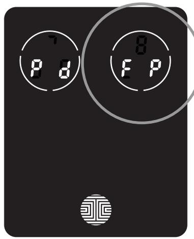
While in **Programming Mode**, select “**2DE**” to delete a **Fingerprint**. If you are not in **Programming Mode**, please see **Section 3.2** to enter **Programming Mode**.
