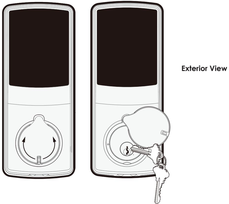
To **unlock** your lock using the **physical key (included)**, open the key cover on the handle by turning the cover to reveal the **keyhole**.
