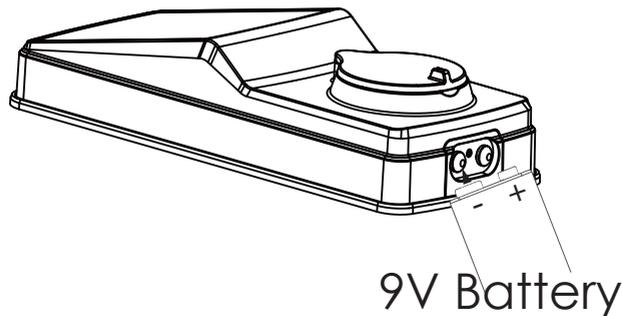
Your Lockly™ will automatically detect battery polarity. So hold your 9V battery lead in place against bottom of the Lockly™ to **temporarily** activate the screen to enter your **Access Code**. Be sure to hold the 9V battery against the contact points located at the bottom of the lock until you have successfully unlocked your door with your **Access Code**. Once unlocked, batteries should be replaced immediately.
