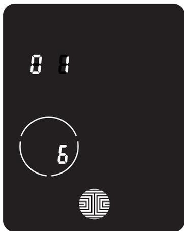
Once you're in **Fingerprint Registration Mode** you will see two numbers displayed on keypad. The top number is your **Fingerprint Registration** number, in this example to the left, **"1"**. The bottom number will always start with a **"6"**.
